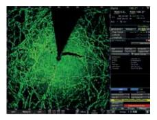
Argus X-Band - ice detection mode showing an open water crack in the ice
