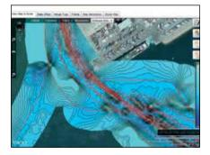
Data Capture - Survey area whilst recording sonar logs
