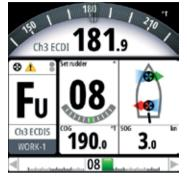
Detailed thruster interface with visual reference of thruster activity
