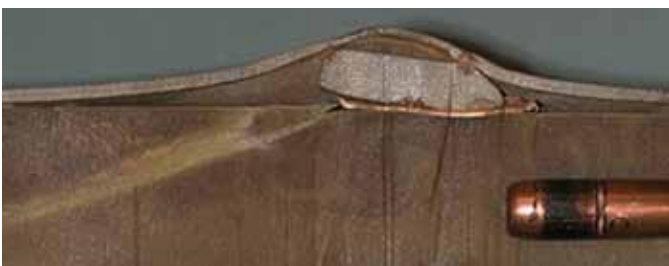
Tests carried out at the UK MoD's Defence Evaluation Research Agency (QinetiQ) showed that SPS stops projectiles at shorter strike ranges and higher angles of attack. SPS reduced risk of penetration by 75% compared with equivalent all steel structure.
