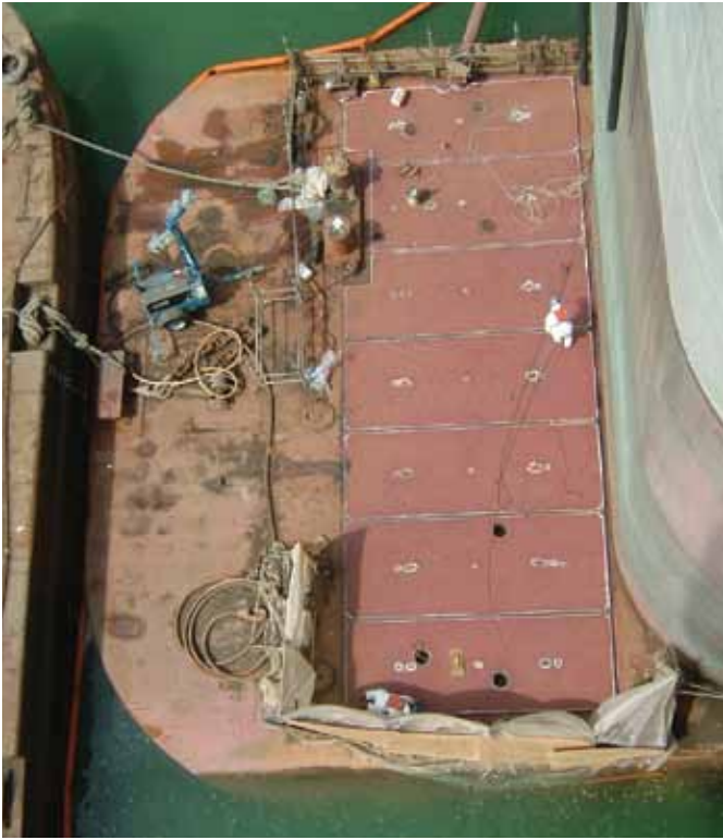
SPS Overlay for pontoons of drilling rig is able to absorb impact of 3 tonne drill collar falling from height of 37 metres without rupture.
