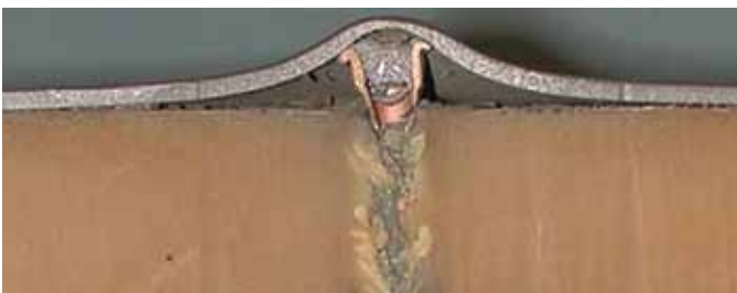
Blast tests carried out at US Navy's Naval Surface Warfare Center (NSWC) demonstrate how SPS absorbs more blast energy, reduces risk of premature rupture and limits fragment penetration. The conventional steel panel (left) is ruptured by the blast while the SPS panel (right) absorbs the energy and deforms without rupture.
