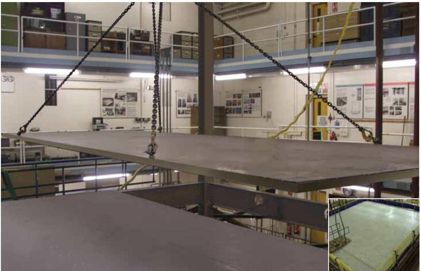
A full-scale 9m x 9m bay, fitted out with M&E, suspended ceilings and raised access floors has been fully tested at the UK Building Research Establishment (BRE). Inset picture shows Techniks ceramic raised floor system installed on SPS panels
