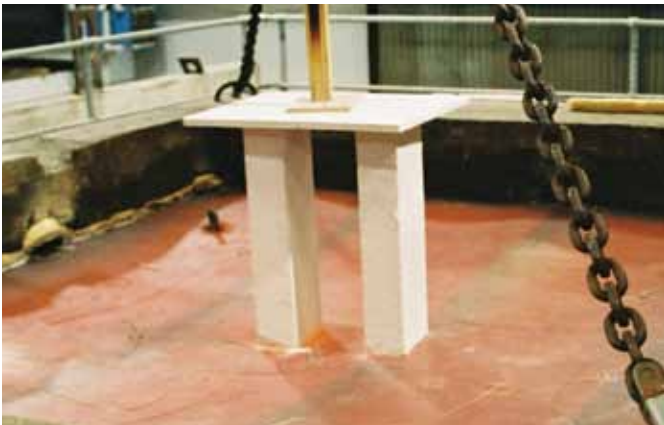
Tests carried out at the Danish Institute of Fire Technology (DIFT) show un-insulated steel structure red hot (left) after 60 minutes at 945°C vs. maximum temperature for SPS of 38°C (note the bare feet).
