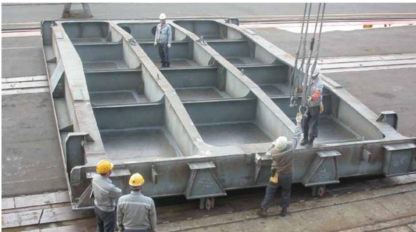
SPS hatch cover at DSME shipyard
