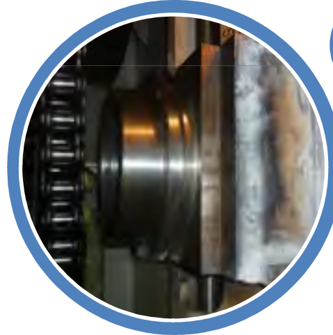
Crack repairing on A-frame
